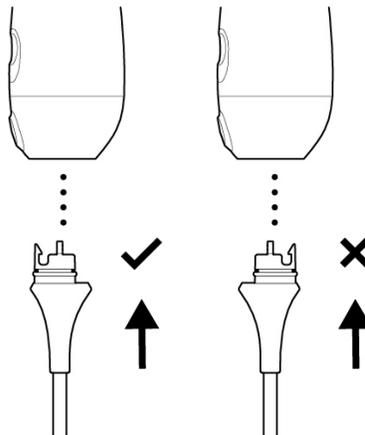
**Figure 7. Expected gap between the cable strain relief and probe body after installing the Butterfly iQ3 cable**
