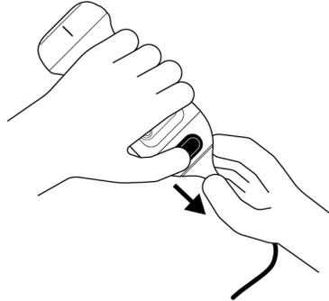
2. Align the connector and the probe, and push the cable firmly into the probe body. When the cable is fully installed, you will feel a light “click” when the cable lock feature on the probe engages with the cable.
